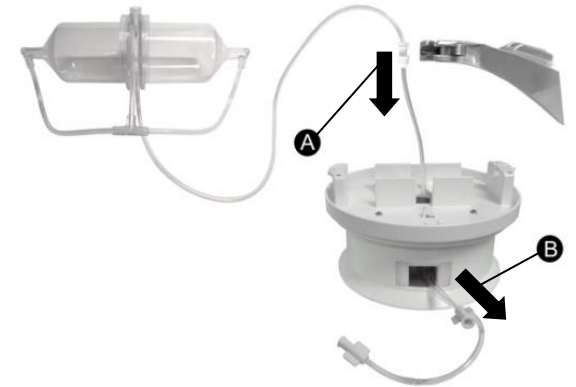
Figure 2. Thread the separation chamber tubing through the center of the chamber caddy.
